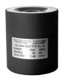
The conversion of measured load is realized due to a steel spring element with strain gage full bridge. The bridge is balanced and thermal compensated. Conversion elements are closed in a hermetic housing which is secured against corrosion with powder lacquer.
